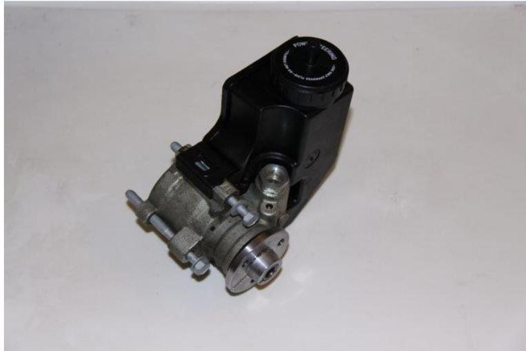
Photo #6 (Pump Mounting Bolts installed into Housing)
