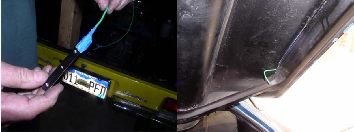
11) Install the small 6-32 screw through the sheet metal into the nut plate bracket. Start the (3) ¼-20 screws to make sure the holes line up, and then tighten the small 6-32 screw. Remove the (3) ¼-20 screws and reinstall through the deck lid mount plate bracket. Pull the wire free and remove.
