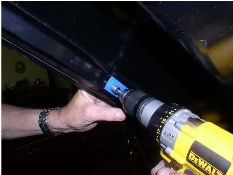
10) Attach the nut plate bracket to a stiff wire with masking tape so that the bracket will line up with the holes. When attaching the wire make sure that the wire is not going to be pinched between the sheet metal and bracket when screws are tighten. Push the bracket up with the wire until it lines up with the drilled holes.
