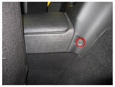
Remove the 2 rear screws (have large flat washer and are slightly larger than the forward screws)
