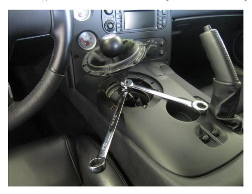
Place the 3/4" wrench on the retaining nut and the 17mm" (for OE shift knob) on the bottom of the shift knob
