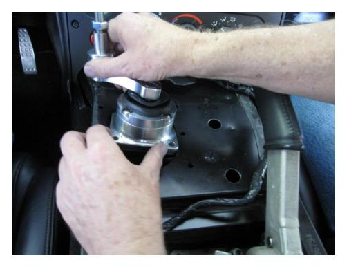
Place the STS into the transmission tunnel and position it over the transmission tail shifter housing
