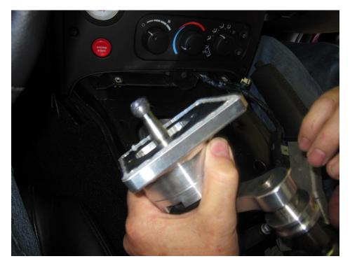
Apply grease to the STS shifter stem ball Apply Loctite RTV silicone (supplied) to the outer mating surface on the STS
