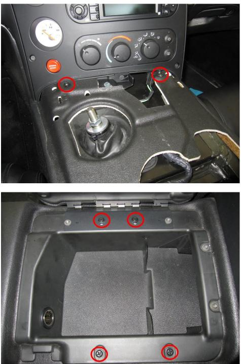
Attach the center console with the 2 forward screws, 2 rear screws and 4 console box screws
