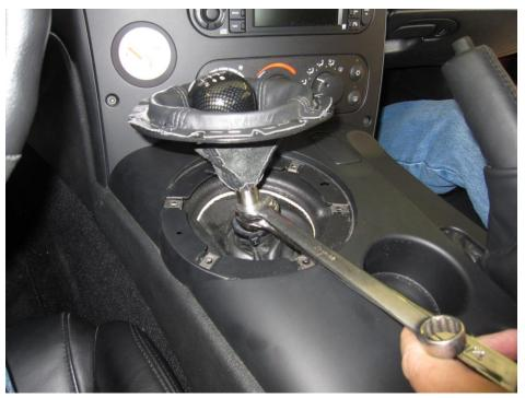
Place the 3/4" wrench on the retaining nut and the 17mm" (for OE shift knob) on the bottom of the shift knob
