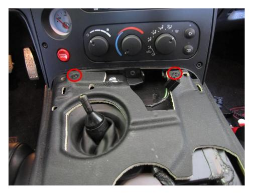
Remove the 2 forward screws Move both seats to their most forward position Position both seatbacks to their most forward position
