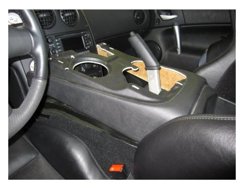
Carefully pull out the front ears of the center console around the center instrument panel bezel
