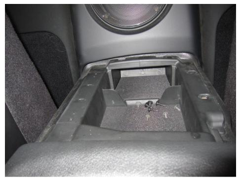
Lift the front of the center console over the parking brake and pull the rear away from the rear bulkhead
