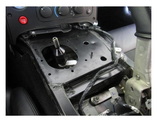
Drill the final holes in the transmission tunnel using a 3/4" bit (or a step bit)
