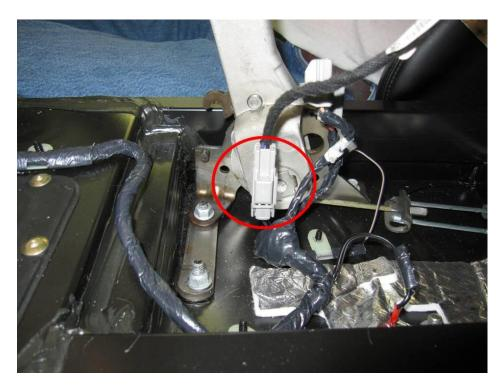
Disconnect the rear accessory power outlet at the connection point (12" down the wire) Lift the front of the center console up over the dash Remove the center console
