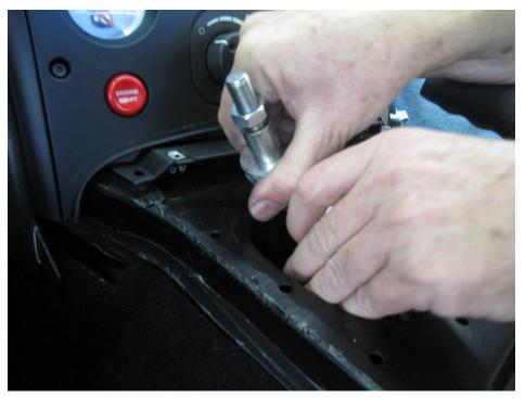
Insert the shifter stem ball of the STS into the transmission shifter receiver
