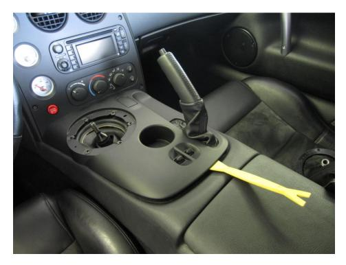
Use the pry tool to remove the console shifter bezel
