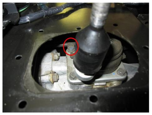
Push aside the connector that is kept down by the forward passenger side cover mounting bolt
