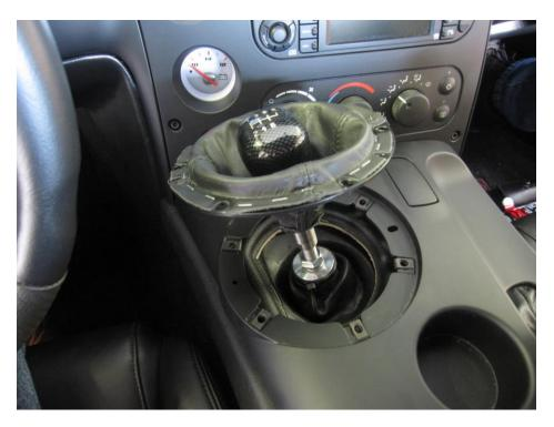
Screw down the shift knob with the upper shift boot attached \*Note: An aftermarket shift knob was installed during this installation.\*
