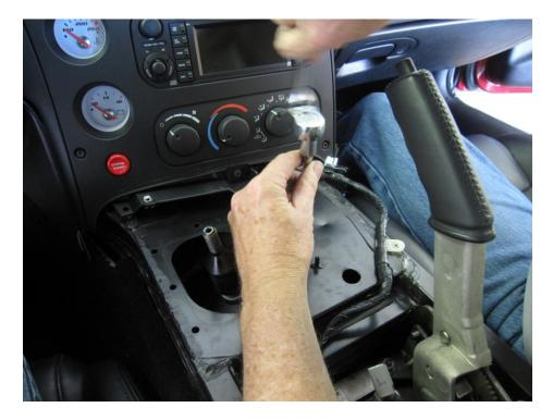
Remove the 4 shifter cover mounting bolts holding the shifter with a socket ratchet, 13mm socket, extension and universal joint
