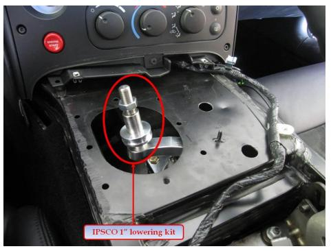
Align the 4 holes and apply a small drop of Red or Blue Loctite to the threads of the new shifter cover mounting bolts (supplied)
