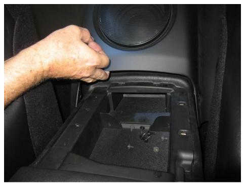
Pull the bottom of the rear bulkhead forward to release the rear of the center console
