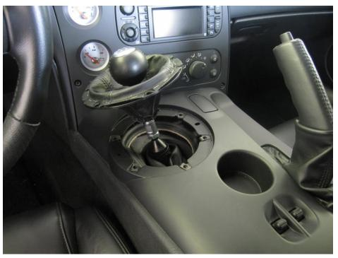
Invert the upper shift boot towards the shift knob to gain access to the retaining nut
