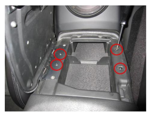
Remove the 4 screws inside the console box (do not remove the 4 torx screws)
