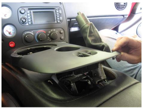
Once the bezel has been pulled away, disconnect the electrical connections Mark the widow switches L (left) and R (right)
