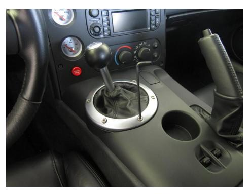
Remove the 6 socket head cap screws from the bezel ring using a 3/16" Allen wrench
