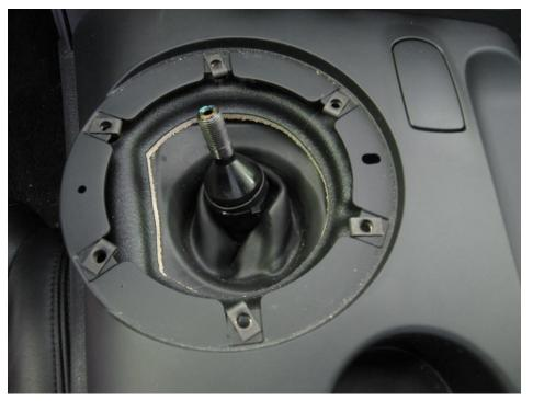
Cut the tie wrap holding the lower shift boot to the isolator
