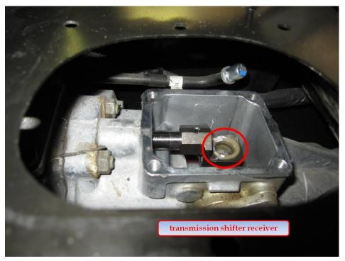
Remove the gasket material from the shifter mating surface on the transmission tail shifter housing with a razor blade Clean all debris out of the transmission tail shifter housing
