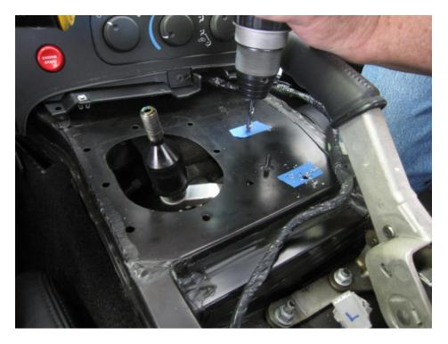
Drill the pilot holes in the transmission tunnel using a 1/4" bit
