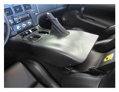
Position the center console so that the parking brake handle will pass through its boot in the console
