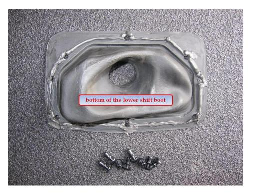
Apply Loctite RTV Silicone (supplied) to the mating surface on the bottom of the lower shift boot Place the lower shift boot over the shift handle and match up the 8 holes
