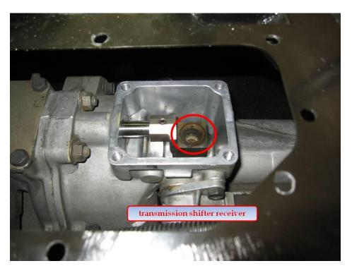
Remove gasket material from the shifter mating surface on the transmission tail shifter housing with a razor blade
