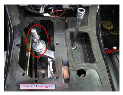
Align the 4 holes and apply a small drop of Red or Blue Loctite to the threads of the new longer shifter cover mounting bolts (supplied) Insert the new shifter cover mounting bolts into each corner Start with the 2 easily accessible corners (driver side) \*Note: An IPSCO 1" lowering kit was also installed during this installation\*
