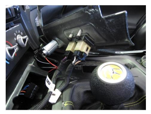
Connect the electrical connections: window switches, cigar lighter and rear defrost switch (GTS only)
