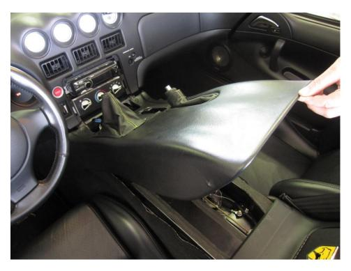
Lift the rear of the center console up; passing the parking brake handle through the its boot and the upper shift boot
