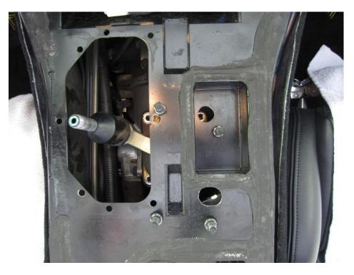
Remove the 4 shifter cover mounting bolts holding the shifter with a socket ratchet, 13mm socket, extension and universal joint (if needed)
