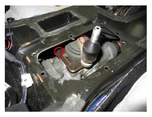
2 of the shifter cover mounting bolts aren't easily accessible They can be removed by drilling access holes just above them in the transmission tunnel
