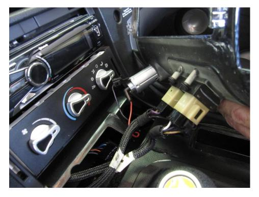
Once the bezel has been pulled away, disconnect the electrical connections: window switches, cigar lighter and rear defrost switch (GTS only) www.ipsco.org – Elizabeth, Colorado – 303-252-4481
