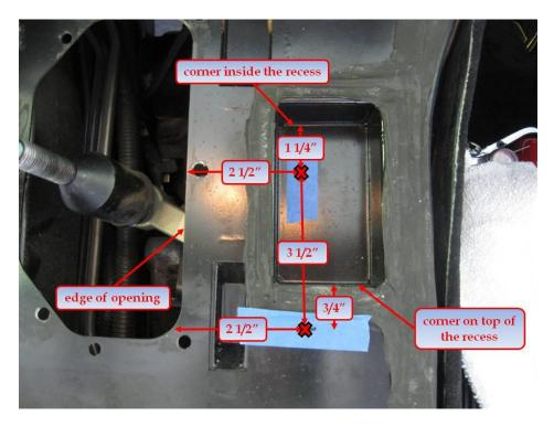
Mark the 2 spots, one inside the ash tray recess and one on top of the transmission tunnel Visually inspect where the marked spots are making sure they are above the 2 shifter cover mounting bolts
