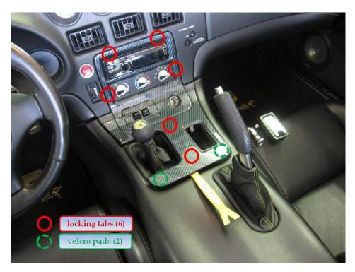
Remove the cigar lighter Remove the ash tray Raise the parking brake handle to its most upright position Use the pry tool to break loose the 2 velcro pads and 6 locking tabs
