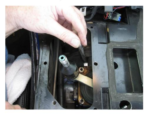
Use the small pry bar to break the original shifter away from the transmission tail shifter housing Lift the original shifter up and away from the transmission tail shifter housing and slip it though the opening
