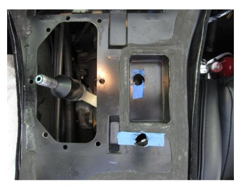
Use a hammer and punch in both marked spots to make an indention so that the drill bit won't travel
