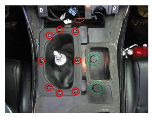
Attach the lower shift boot using the supplied push-in nylon rivets (supplied) Position the boot opening around the isolator of the OE shift shaft (in this case, the lower shift boot 1" lowering kit collar; use the tie wrap (supplied with that kit) to tighten the boot to the lower shift boot collar)
