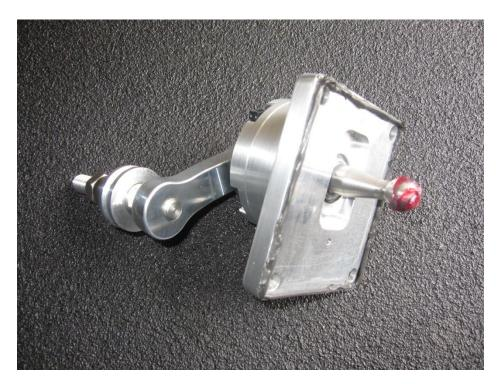
Apply grease to the STS shifter stem ball
