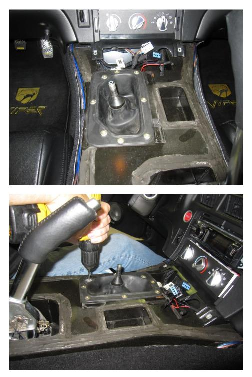
Drill out the rivets (8) using a 1/4" bit The rivets will want to rotate while drilling them out, use vise grips to keep the rivets from turning to minimize the damage to the lower shift boot
