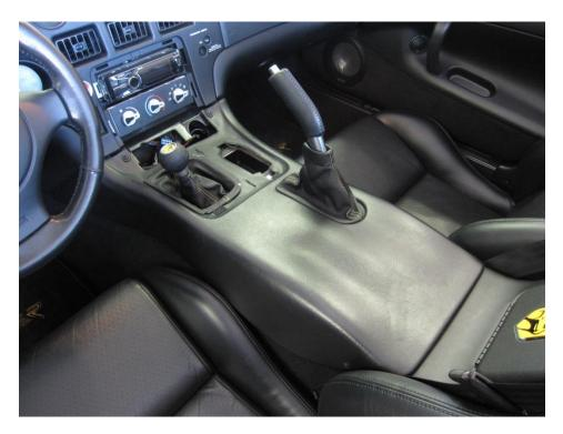
Push the upper shift boot down past the retaining nut Screw the shift knob onto the STS shifter handle Screw the retaining nut to the desired height Use the 3/4" and 5/8" wrenches to tighten the shift knob to the retaining nut Pull the upper shift boot up over the retaining nut to the desired height
