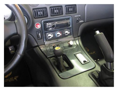
Turn the A/C knobs to the horizontal position
